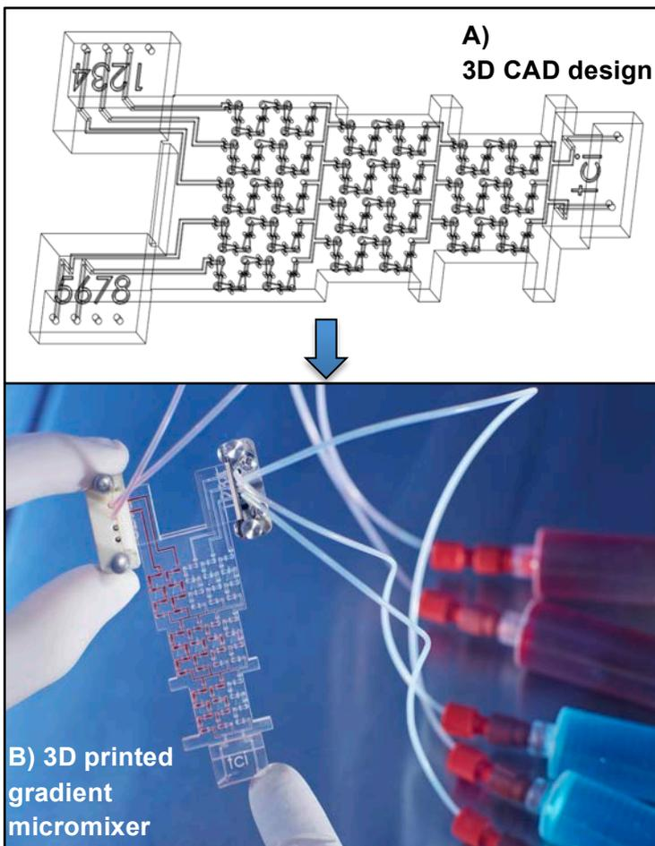
**Fig. 2: From 3D design to 3D printing:** A) 3D-CAD (Computer-aided design) of a tree-shaped gradient micromixer. B) The 3D printed tree-shape gradient micromixer that allows for the rapid mixing of solutions in order to achieve a defined concentration gradient at the outlets of the device.
